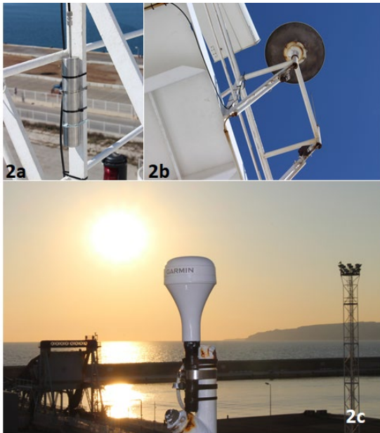
Figure 25. View of air inlet (2a and 2b) and GPS sensor (2c)
