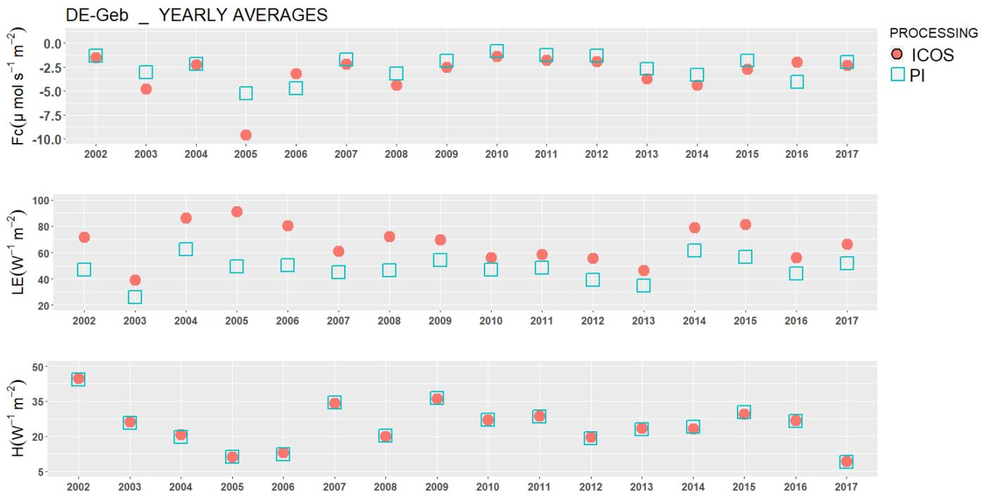
Note: in 2017 the ICOS setup has been implemented. Close path IRGA with 12m tube. PI processing using Eddypro
