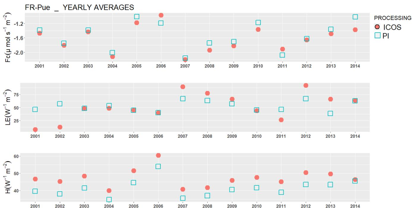
Note: in 2014 the ICOS setup has been implemented. Close path IRGA with 3.5m tube. PI processing using Eddypro
