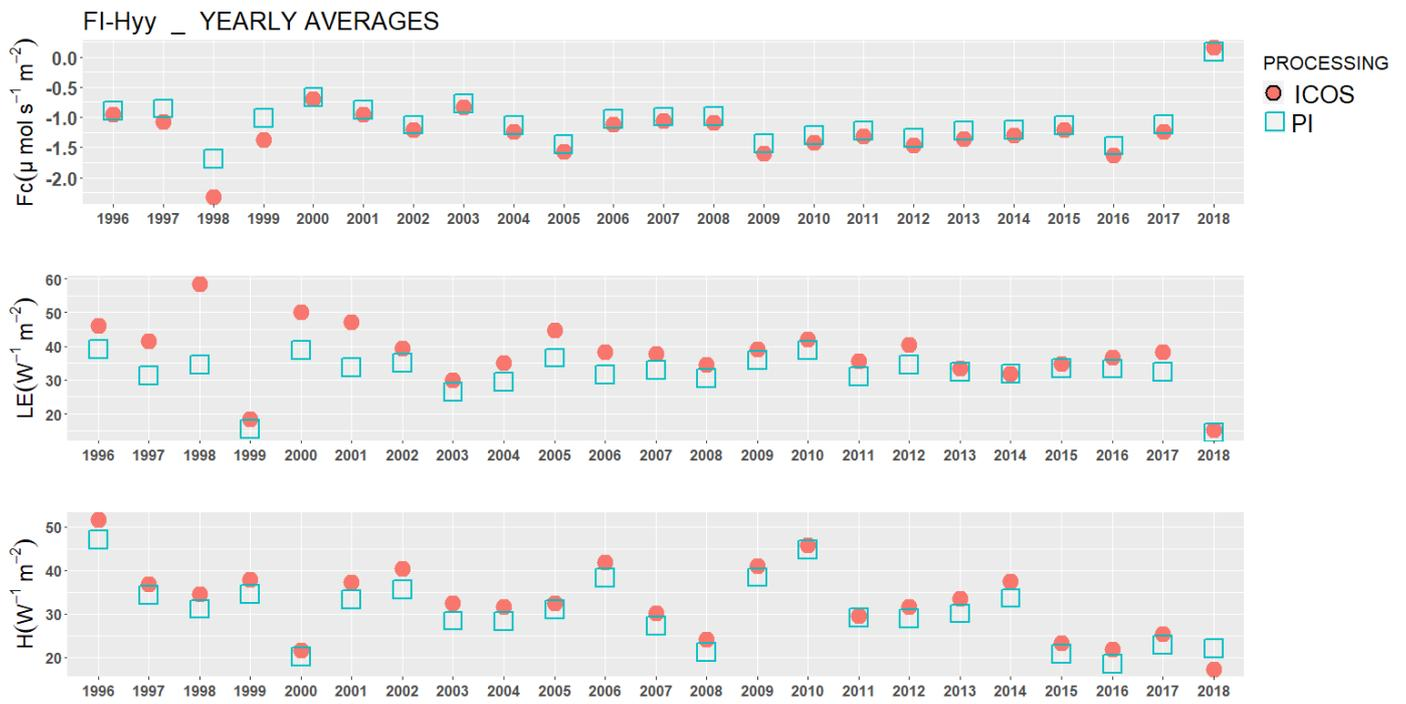
Note: in 2018 the ICOS setup has been implemented. Close path IRGA with 8m tube. PI processing using EddyUH
