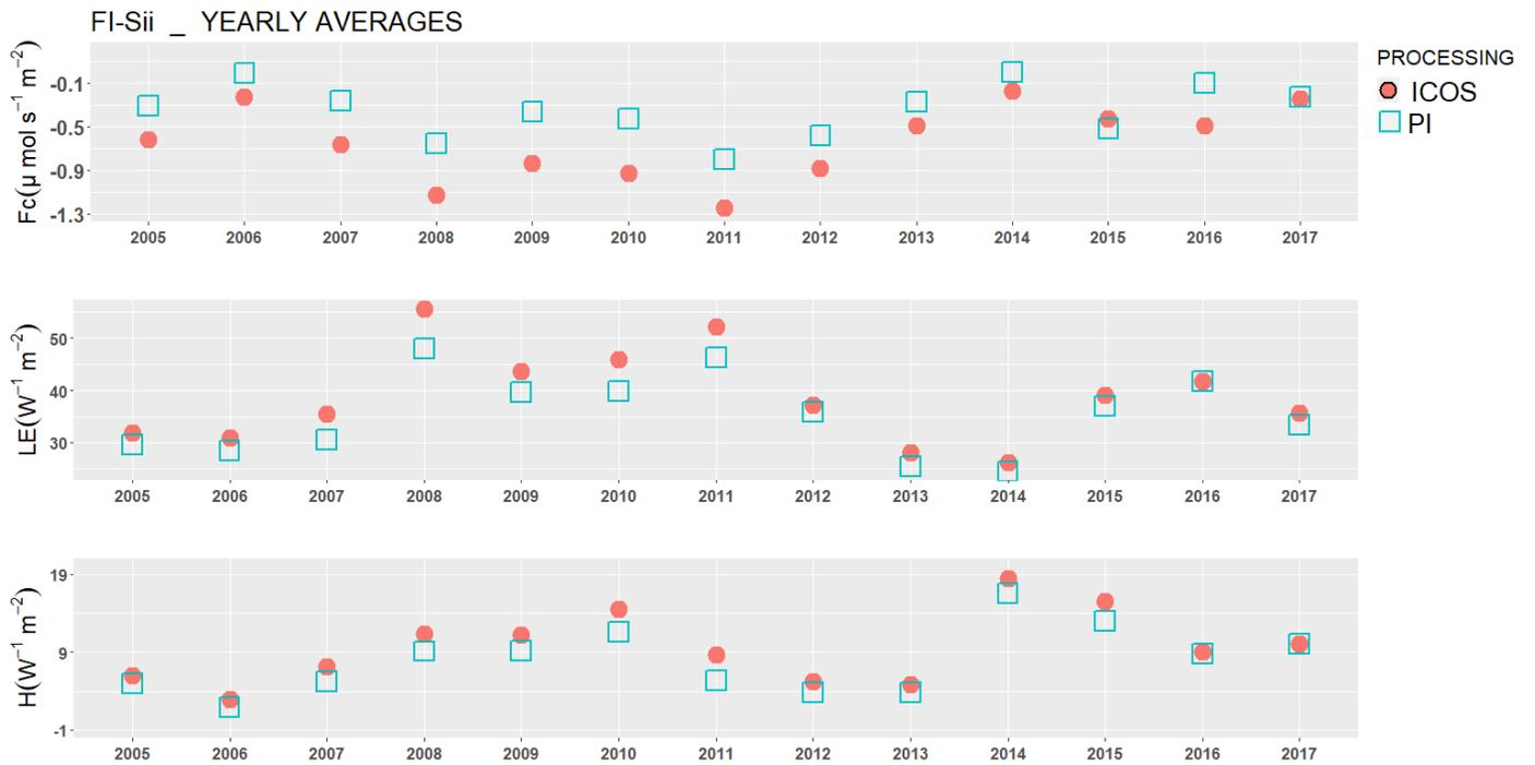
Note: in 2015 the ICOS setup has been implemented. Close path IRGA with 13m tube. PI processing using EddyUH
