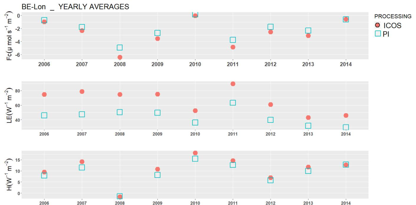
*Note: in 2014 the ICOS setup has been implemented. Close path IRGA with 12m tube. PI processing using Eddysoft*
