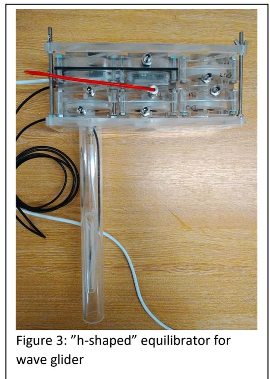
Figure 3: “h-shaped” equilibrator for wave glider
