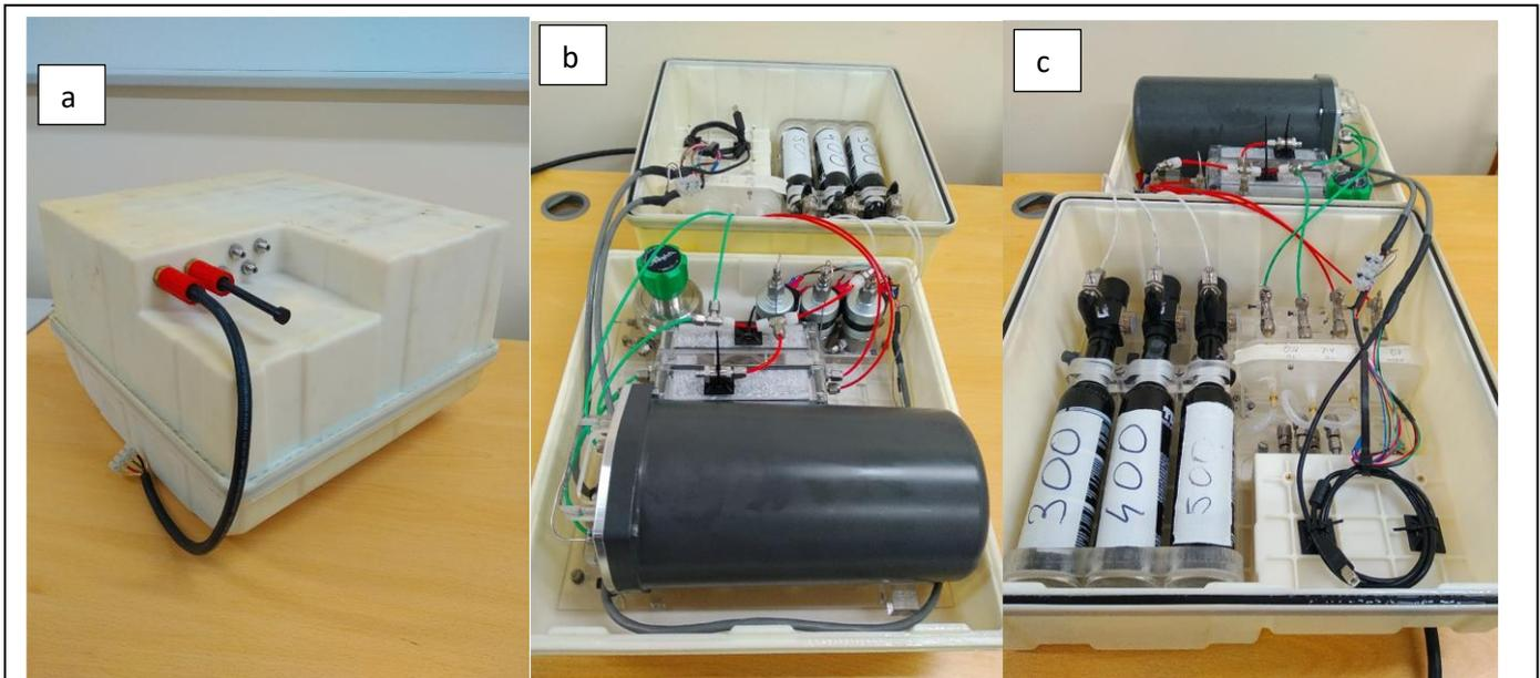
Figure 4: The instrument configured for waveglider: (a) assembled cargo box, (b, c) two views of the opened cargo box.
