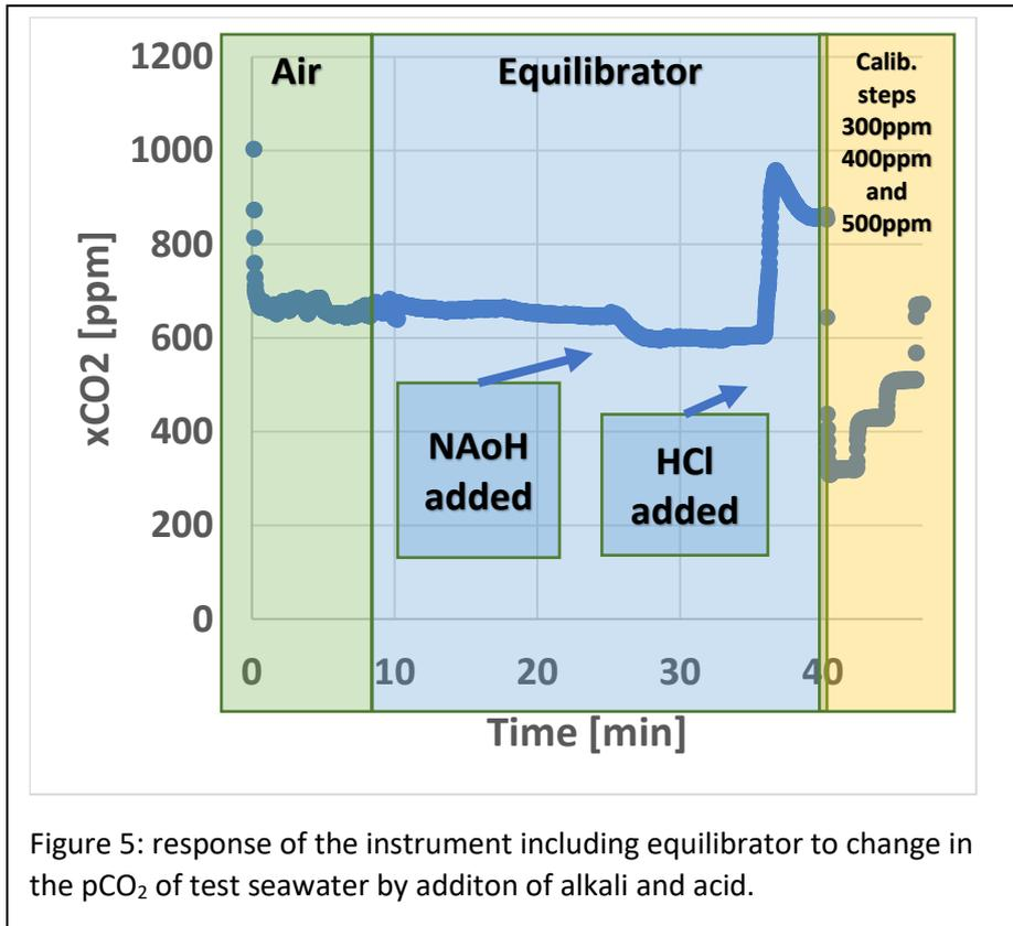
Figure 5: response of the instrument including equilibrator to change in the pCO<sub>2</sub> of test seawater by addition of alkali and acid.
