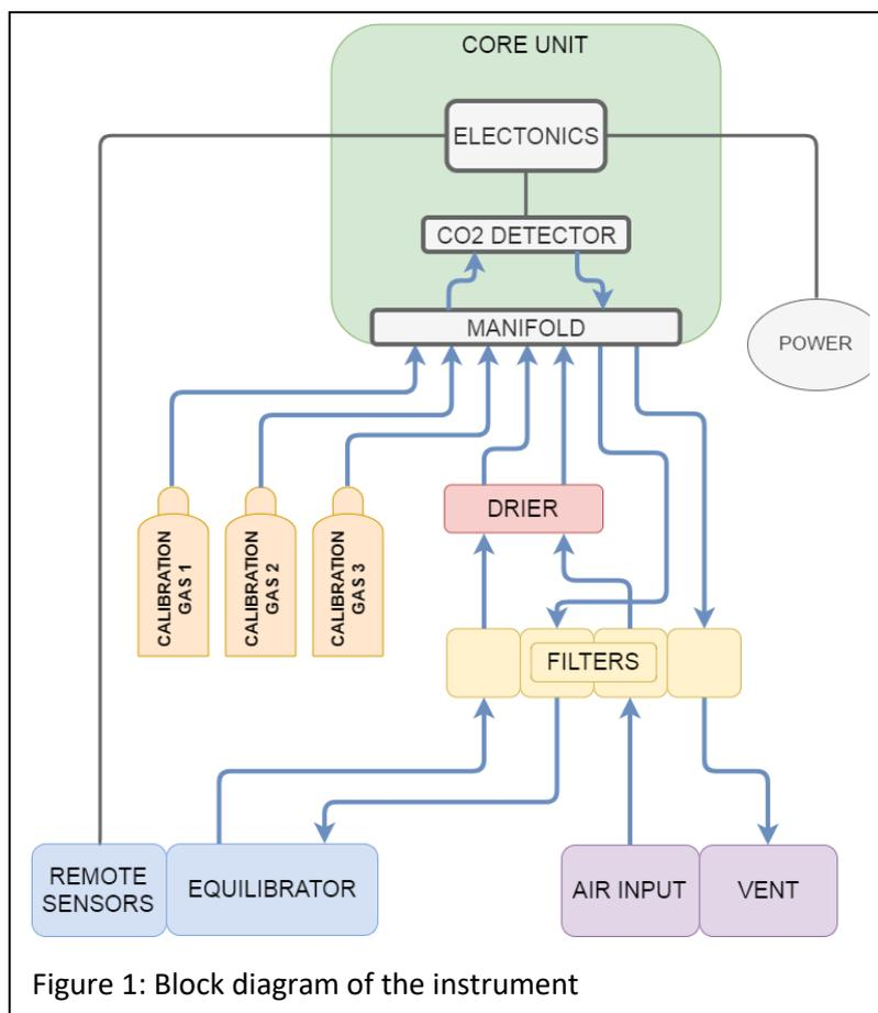
Figure 1: Block diagram of the instrument
