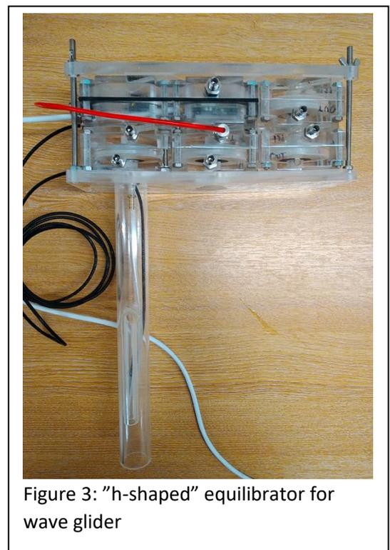
Figure 3: “h-shaped” equilibrator for wave glider
