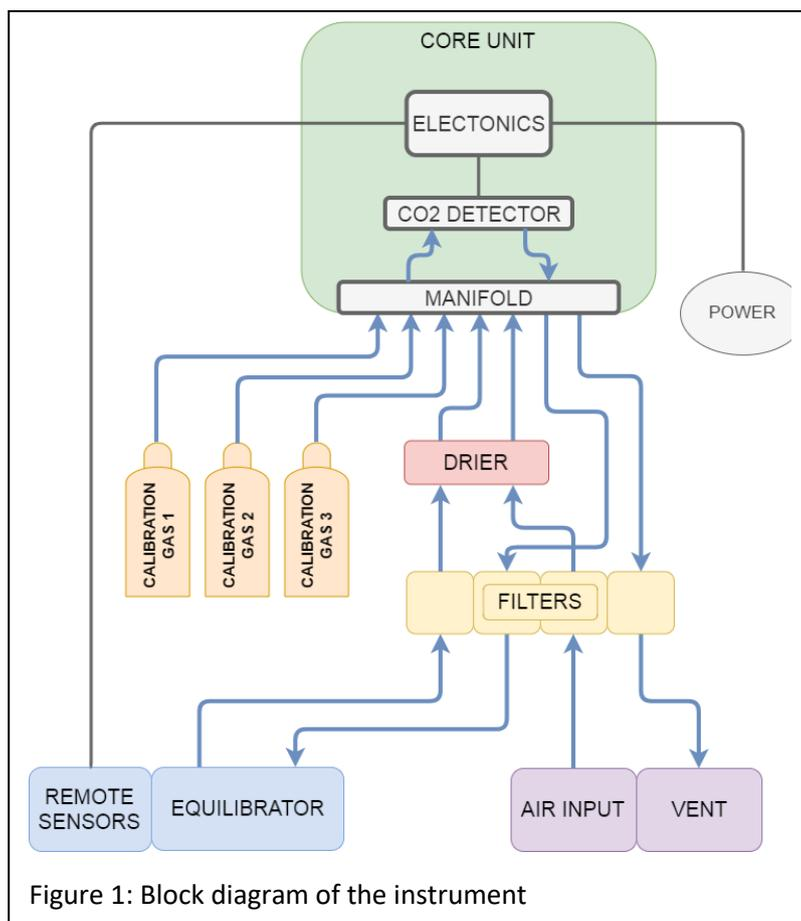
Figure 1: Block diagram of the instrument
