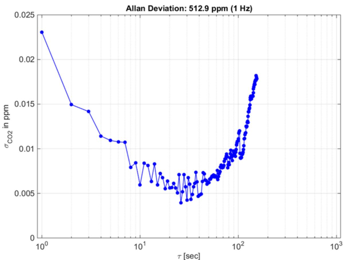
**Figure 8:** Allan deviation analysis of standard gas (512.9 ppm CO<sub>2</sub>) measurement with the LI7815. Measurements were recorded at 1Hz.
