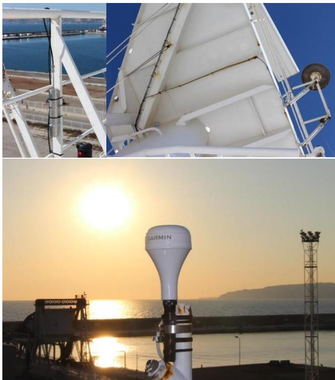
**Figure 11:** View of air inlet (top left and right) and GPS sensor (bottom).
