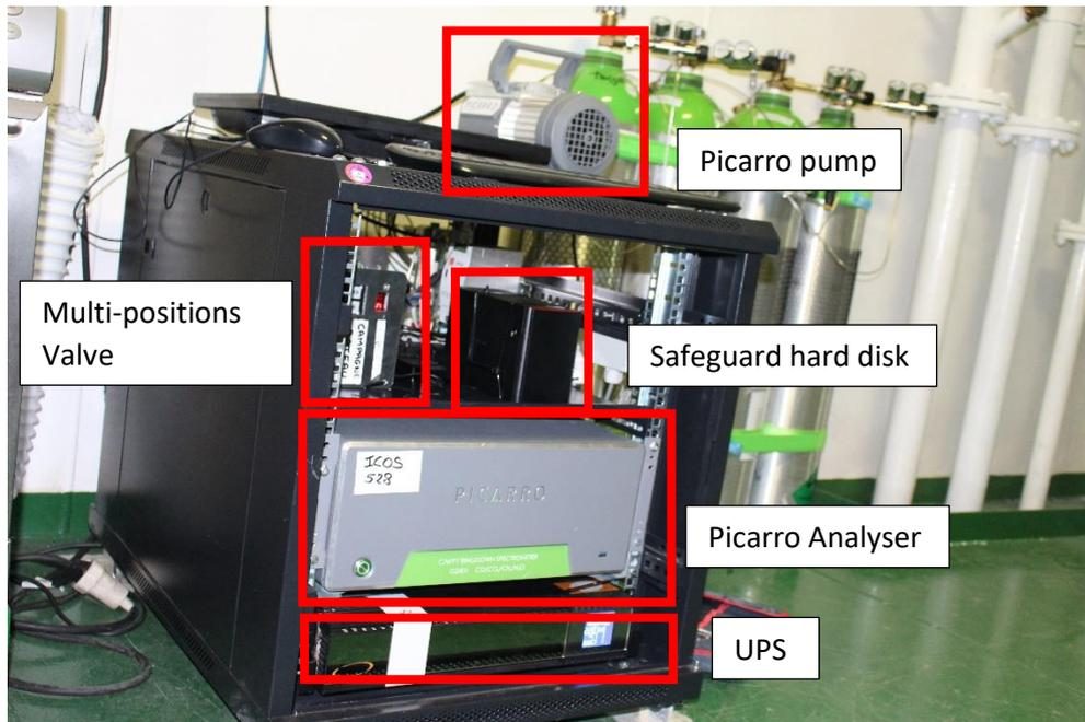
**Figure 10:** Photo of the instrumental set up on the SOOP COLIBRI.
