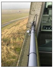
Figure 5: The filtering funnel on the air inlet
