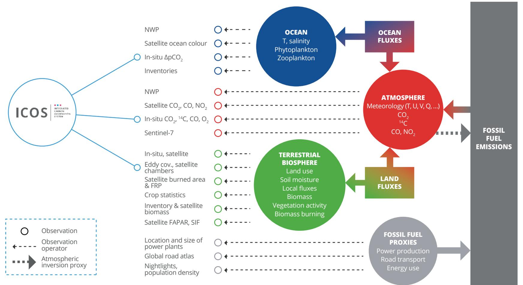
**Figure 4.** ICOS observations related to the schematic overview of a fossil fuel emission inversion system showing the various required model blocks as well as the potential observations that can be used to constrain the system. (From Pinty et al., Copernicus 2017 CO<sub>2</sub> Report)
